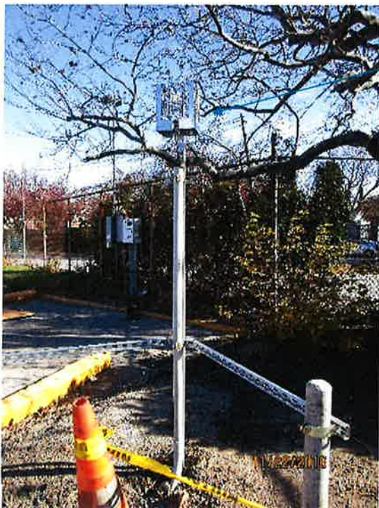
Photograph 2 – Solar powered wet sensor electronic housing
